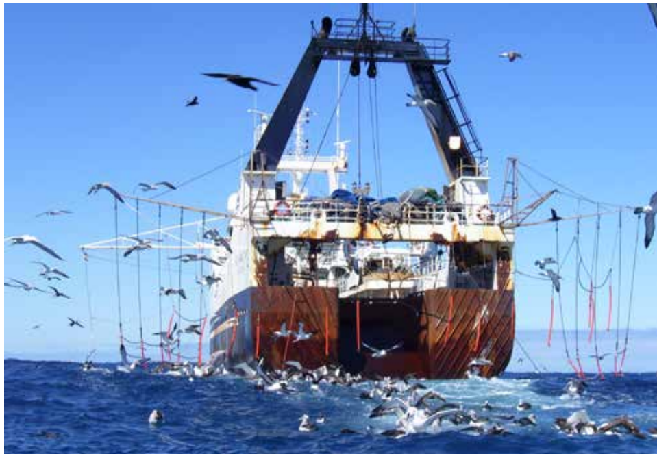
Figure 6.6 On trawl vessels, bafflers create a 'fence' around the stern of a vessel, which keeps the seabirds at a distance so they are unlikely to crash into steel cables.
