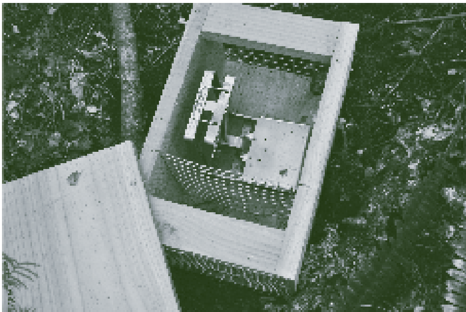
Figure 7.1: Kill traps are designed to quickly kill specific pest species. They are set under covers to stop non-target animals getting killed in the trap.
